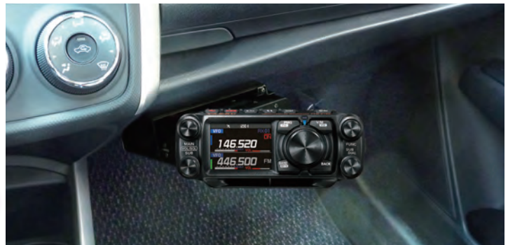
Swing-head kit: SJKM-500 (Optional) Installation Image
