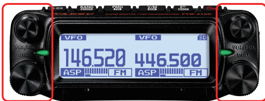
Dial knobs and LED Indicators for each band are placed independently on the left and right side
